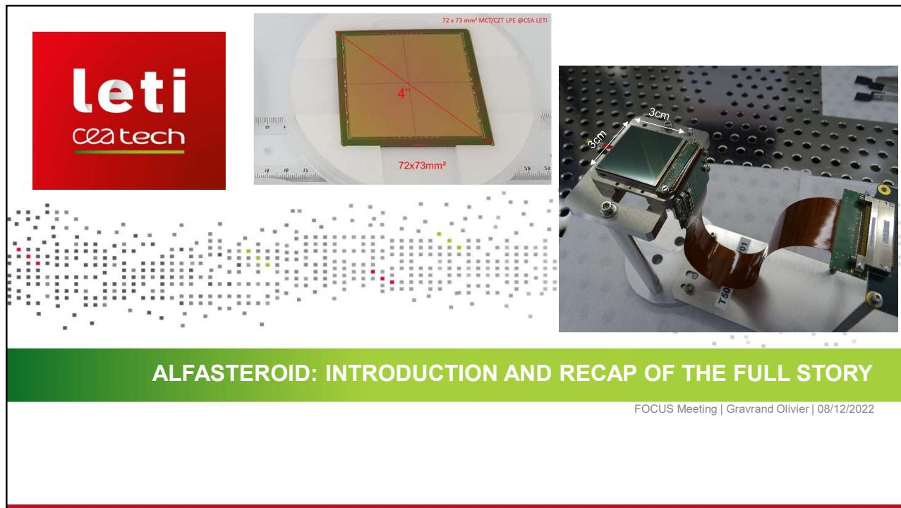
The top section features the Leti CEA Tech logo in red. To its right are two images: one showing a 72x73 mm<sup>2</sup> MCT/CZT LPE detector chip on a circular scale, and another showing the detector mounted in a mechanical assembly with dimensions of 3cm indicated.
